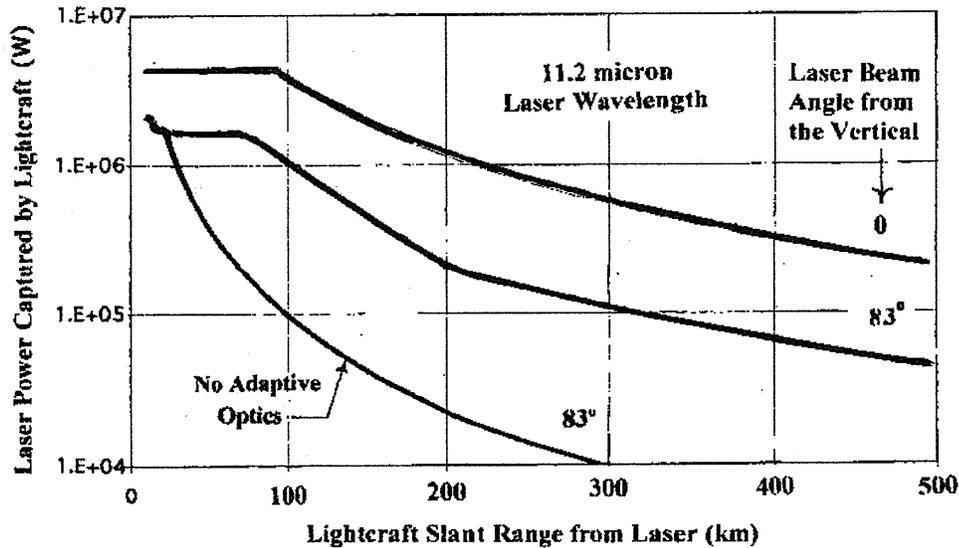
**Figure 12. Captured Laser Power vs. Increasing Range from 11.2  $\mu\text{m}$  CO<sub>2</sub> Laser [26].**
