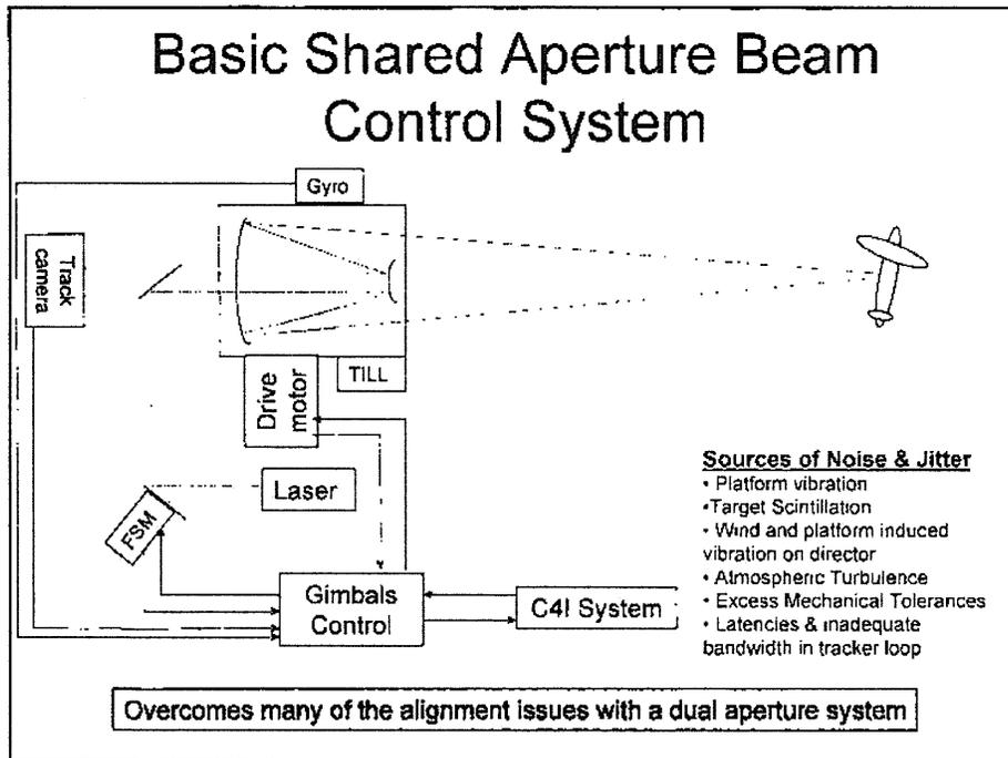
**Figure 35. Basic Shared Aperture Beam Control System (TILL = Track Illuminator Laser; C4I = Command, Control, Computing, Communication & Intelligence equipment) (courtesy of the Directed Energy Professional Society).**
