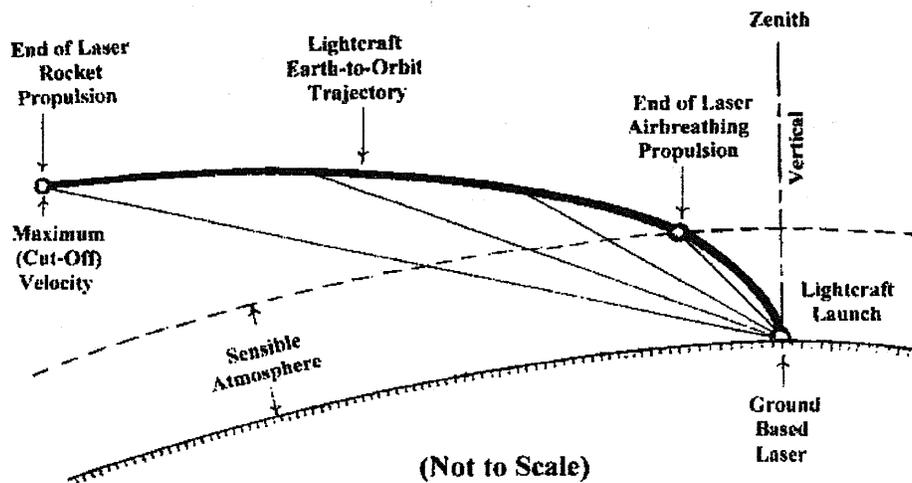
**Figure 8. Lightcraft Trajectory and Associated Pointing Angles** [26].
