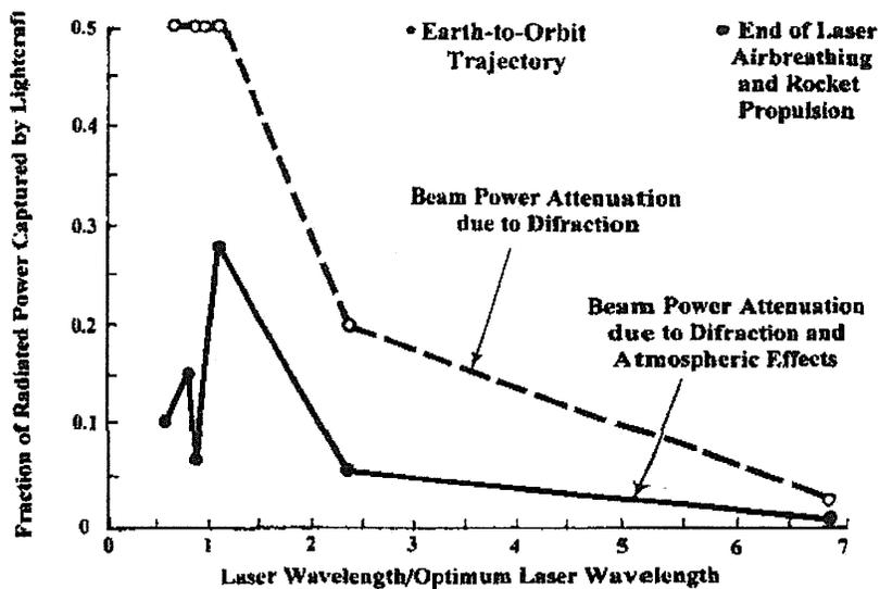
Figure 10. Attenuation Effects on Captured Laser Beam Power [26].
